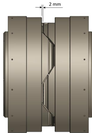
Figure 5-7 HOTDOCK – Max gap before locking.
